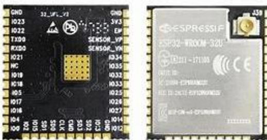
Fig.5 Microcontrolador ESP32-WROOM-32
